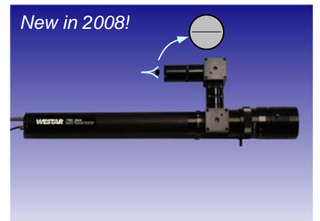
TRD-100A-SAO-STD-STD (direct view optics and adjustable focus)
